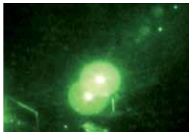
Image intensification: image is saturated by looking directly to a light source.
