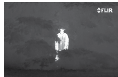
Thermal imaging: suspect hiding in bushes is clearly visible since thermal contrast is practically impossible to mask.
