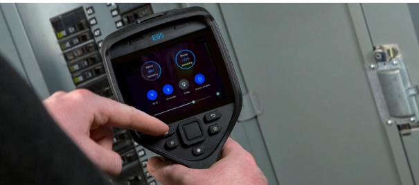
The new Exx-Series is packed with the high performance features you need to quickly find and report hidden hot spots: a bright, bold new screen, razor-sharp lenses, and a rapid-response user interface.
